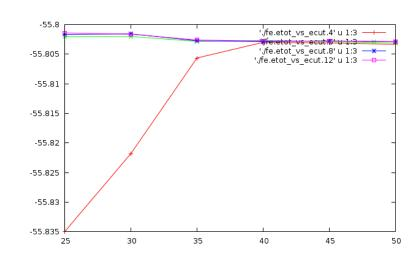
Once convergence is reached for both cutoffs and k-points, you may compare the stability of Iron in the bcc, fcc, hcp phases (the latter being a slightly more complicated structure)
