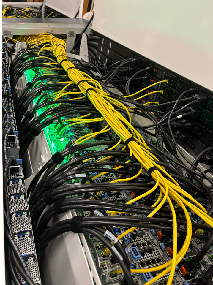
Liquid immersion subsystem by GRC in the Frontera supercomputer at TACC
